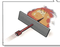
Depleted uranium penetrator with stabilizing fins
